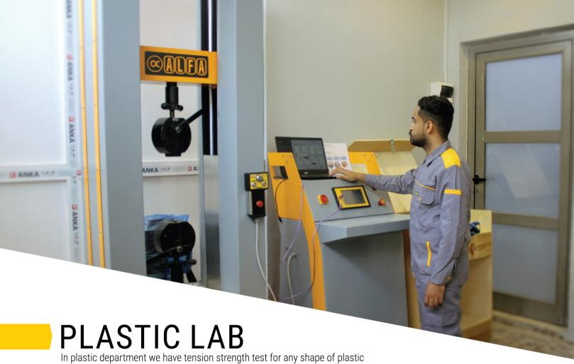
In plastic department we have tension strength test for any shape of plastic and we have test for Geogrid and Geotextile, also we have the following test for plastic pipe
